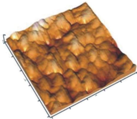
**Figure 5.** AFM scan of implanted fullerenes thin films ( $^{60}\text{C}$ ) by boron ions  $\text{B}^{3+}$  with an irradiation dose of  $D = 2 \cdot 10^{16} \text{ cm}^{-2}$  and kinetic energy  $E = 45 \text{ keV}$ . Image size:  $1.0 \times 1.0 \mu\text{m}^2$
