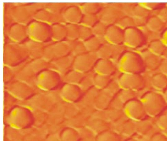
**Figure 3. AFM scan of implanted fullerenes thin films (<sup>60</sup>C) by nitrogen ions  $\text{N}^{2+}$  with an irradiation dose of  $D = 2 \cdot 10^{17} \text{ cm}^{-2}$  and kinetic energy  $E = 30 \text{ keV}$ . Image size:  $1.5 \cdot 1.5 \mu\text{m}^2$**
