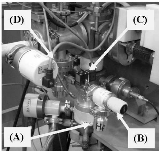
**Figure 1. The modified main gas inlet system of the MIVOC method at the injection stage of mVINIS**
