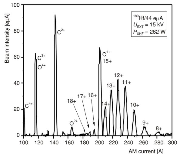
**Figure 2. Spectrum of  $^{180}\text{Hf}$  ions obtained by the MIVOC method**
