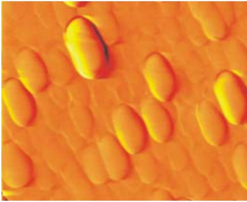
**Figure 4.** AFM scan of implanted fullerenes thin films ( $^{60}\text{C}$ ) by nitrogen ions  $\text{N}^{5+}$  with an irradiation dose of  $D = 2 \cdot 10^{17} \text{ cm}^{-2}$  and kinetic energy  $E = 75 \text{ keV}$ . Image size:  $1.5 \times 1.5 \mu\text{m}^2$
