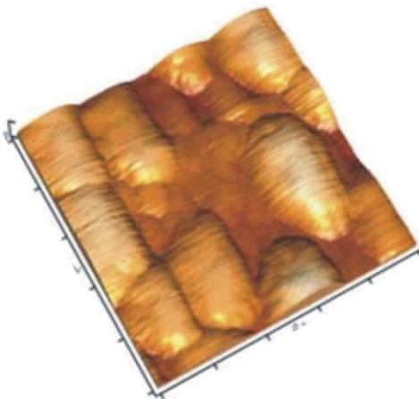
**Figure 6.** AFM scan of implanted fullerenes thin films ( $^{60}\text{C}$ ) by iron ions  $\text{Fe}^{6+}$  with an irradiation dose of  $D = 2 \cdot 10^{16} \text{ cm}^{-2}$  and kinetic energy  $E = 90 \text{ keV}$ . Image size:  $1.0 \times 1.0 \mu\text{m}^2$
