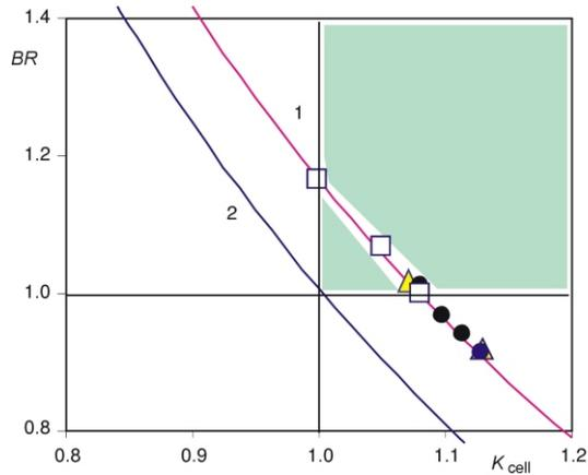
**Figure 3.**  $BR$  values vs.  $K_{cell}$  for heavy water CANDU reactor. Curve 1 – Th-U fuel cycle: ● – cell variant 1 at different lattice pitch (28.6, 23.2, 20.6 cm), □ – cell variant 5, and ▲ – cell variant 2 at different contents of  $^{233}\text{U}$  in thorium. Curve 2 – U-Pu fuel cycle
