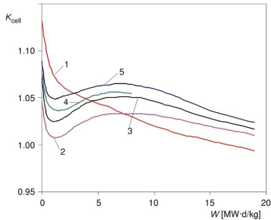
**Figure 5.**  $K_{\text{cell}}$  values vs.  $W$  for different initial content of  $^{233}\text{U}$  in the cell. Curve 1 – 24.1 g/cm, cell variant 1. Curve 2 – 24.1 g/cm, cell variant 2. Curve 3 – 25.3 g/cm, cell variant 2. Curve 4 – 25.7 g/cm, cell variant 2. Curve 5 – 26.5 g/cm, cell variant 2
