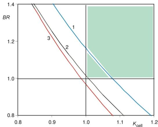
**Figure 4.**  $BR$  values vs.  $K_{cell}$  for light water VVER-1000 reactor. Curve 1 – Th-U fuel cycle and curve 2 – U-Pu fuel cycle without boron, curve 3 – Th-U fuel cycle with boron
