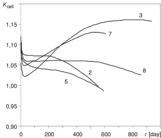
**Figure 1. Multiplication factor  $K_{\text{cell}}$  in operation with constant power during time  $\tau$ . Number of curves corresponds to variants of tab. 1**
