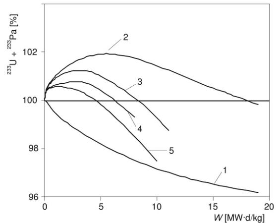
**Figure 6.** Respective amount of  $^{233}\text{U} + ^{233}\text{Pa}$  in the cell vs.  $W$  for different initial content of  $^{233}\text{U}$  in the cell. Designation of curves – as in fig. 5
