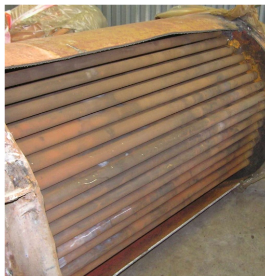
Figure 5. Heat exchanger tubes before segmentation
