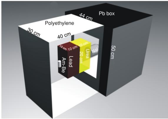
**Figure 1. Schematic set-up of the  $^{241}\text{Am-Be}$  source based PGNAA set-up with the source-inside-moderator geometry**
