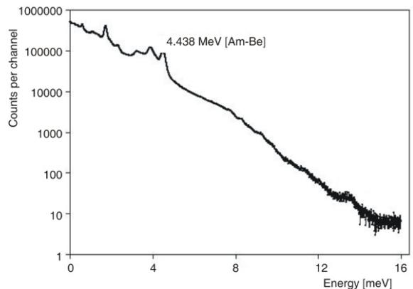
**Figure 10.** Prompt gamma ray spectrum of urea with (f) structure and the cubical Pb shield in front of the neutron source replaced with cubical polyethylene
