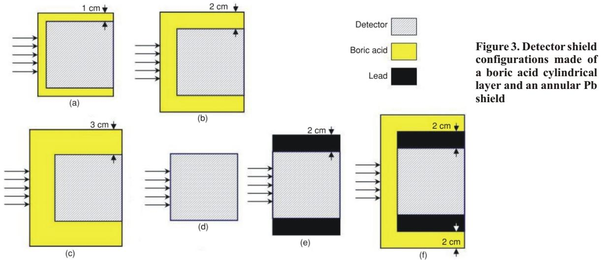
**Figure 3. Detector shield configurations made of a boric acid cylindrical layer and an annular Pb shield**
