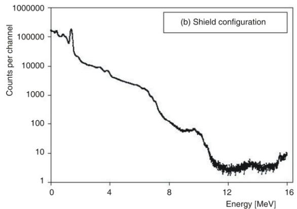
**Figure 5. Prompt gamma ray spectrum of urea with (b) structure**
