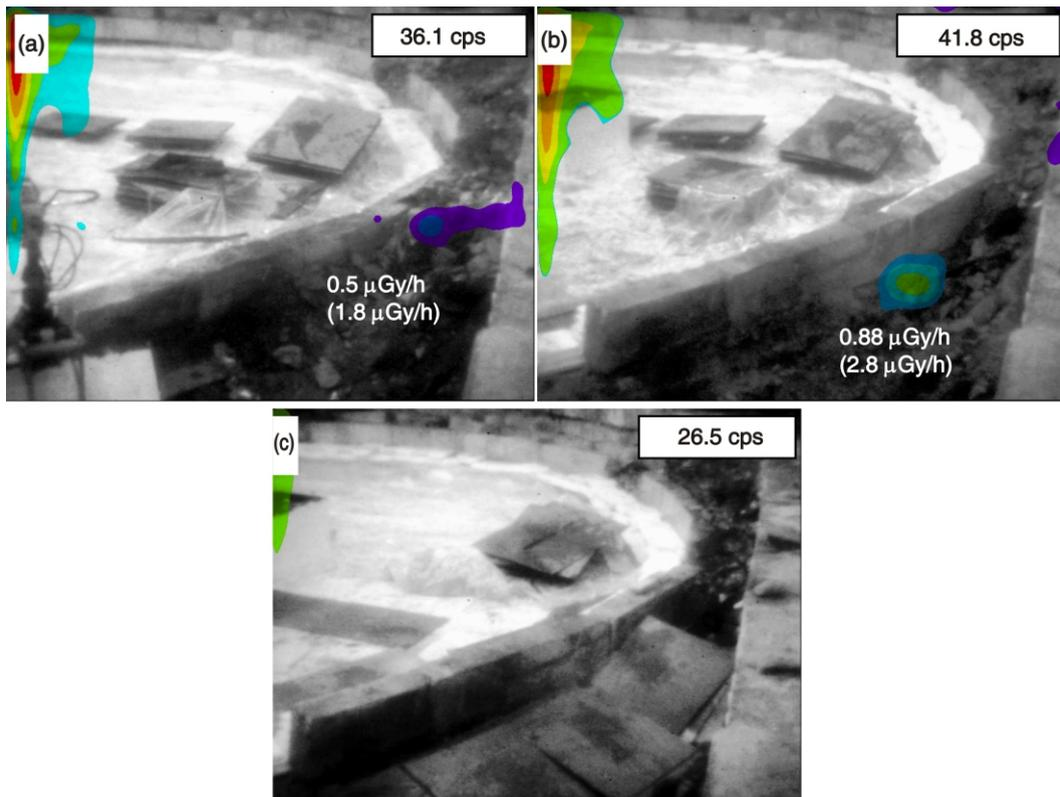
**Figure 7.**  $\gamma$ -dose rates from the source at the side of the DSU 3A tank measured by the CARTOGAM (2011)
