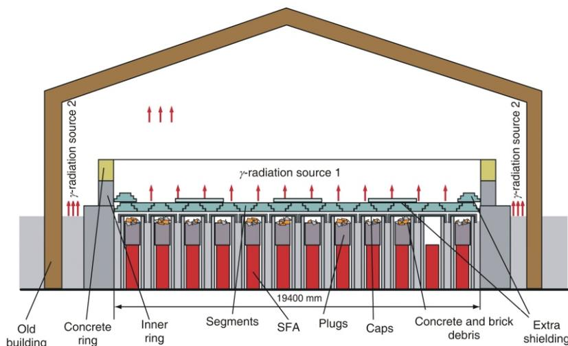
**Figure 2.  $\gamma$ -radiation source at the DSU 3A under the cover (27. 02. 2012)**
