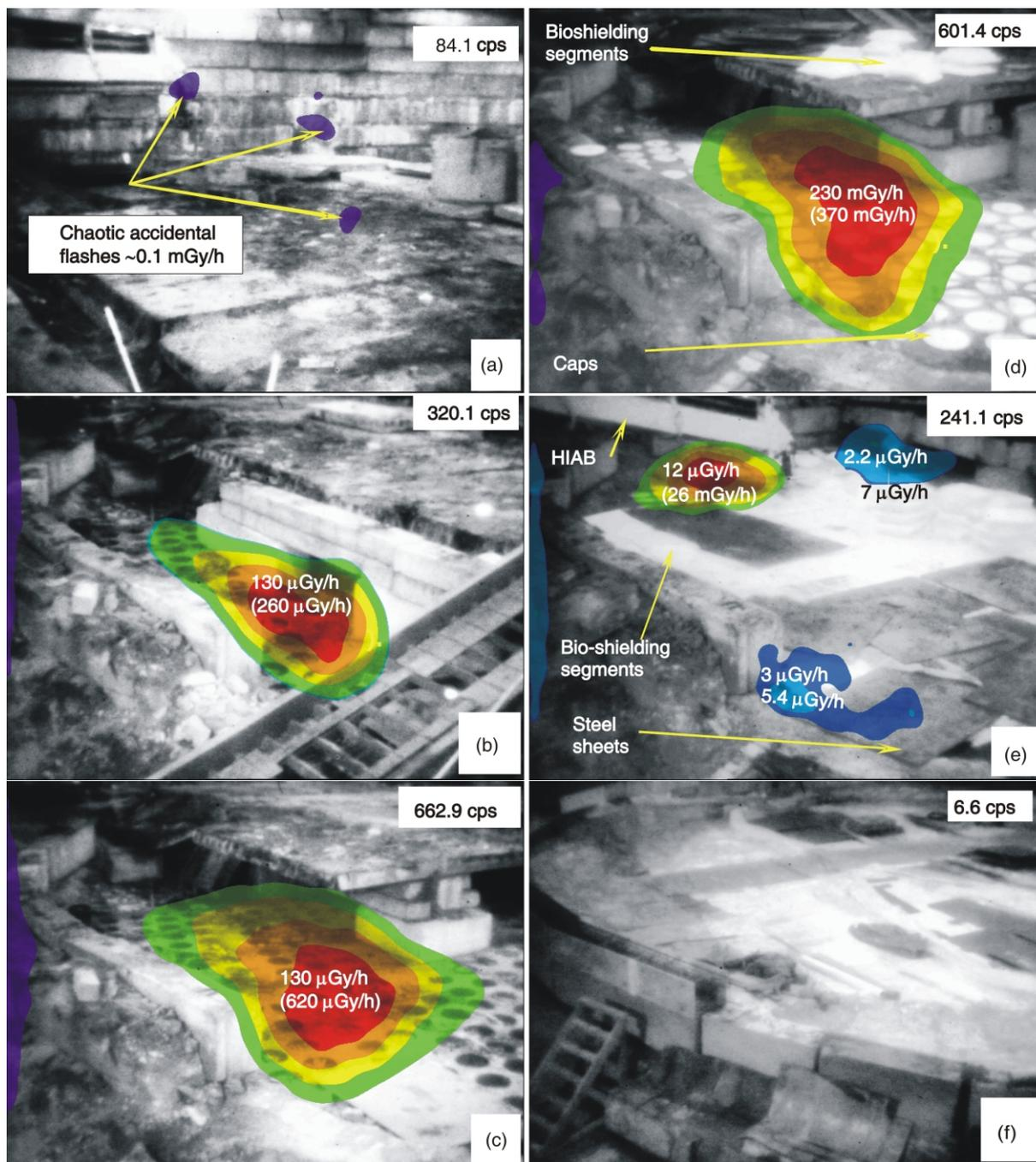
**Figure 6.  $\gamma$ -dose rates from the sources at the DSU 3A surface measured by the CARTOGAM**
