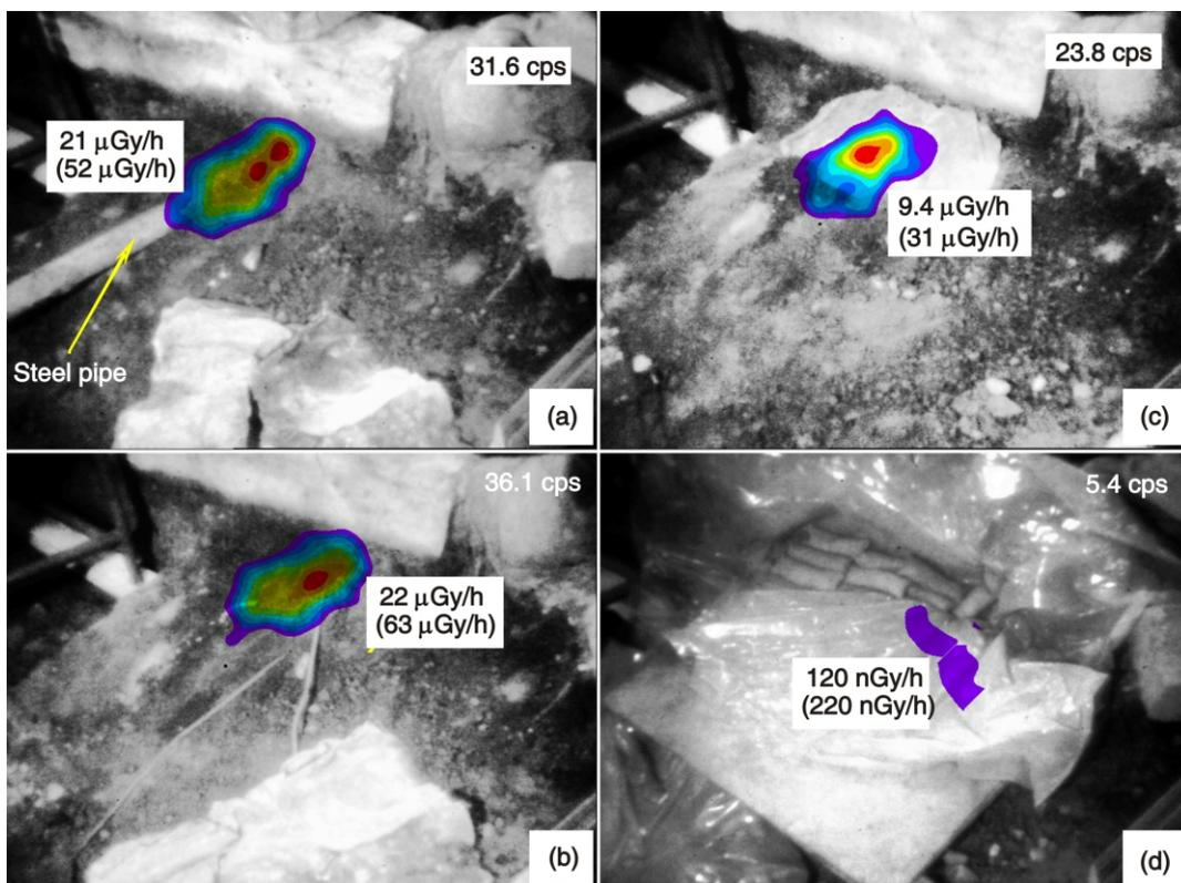
**Figure 8.** An unknown  $\gamma$ -source detected at the entrance to the DSU 3A tank by the CARTOGAM
