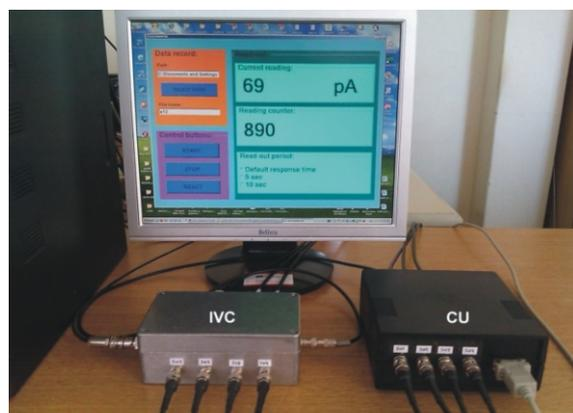
Figure 4. Auto-ranging electrometer in operation
