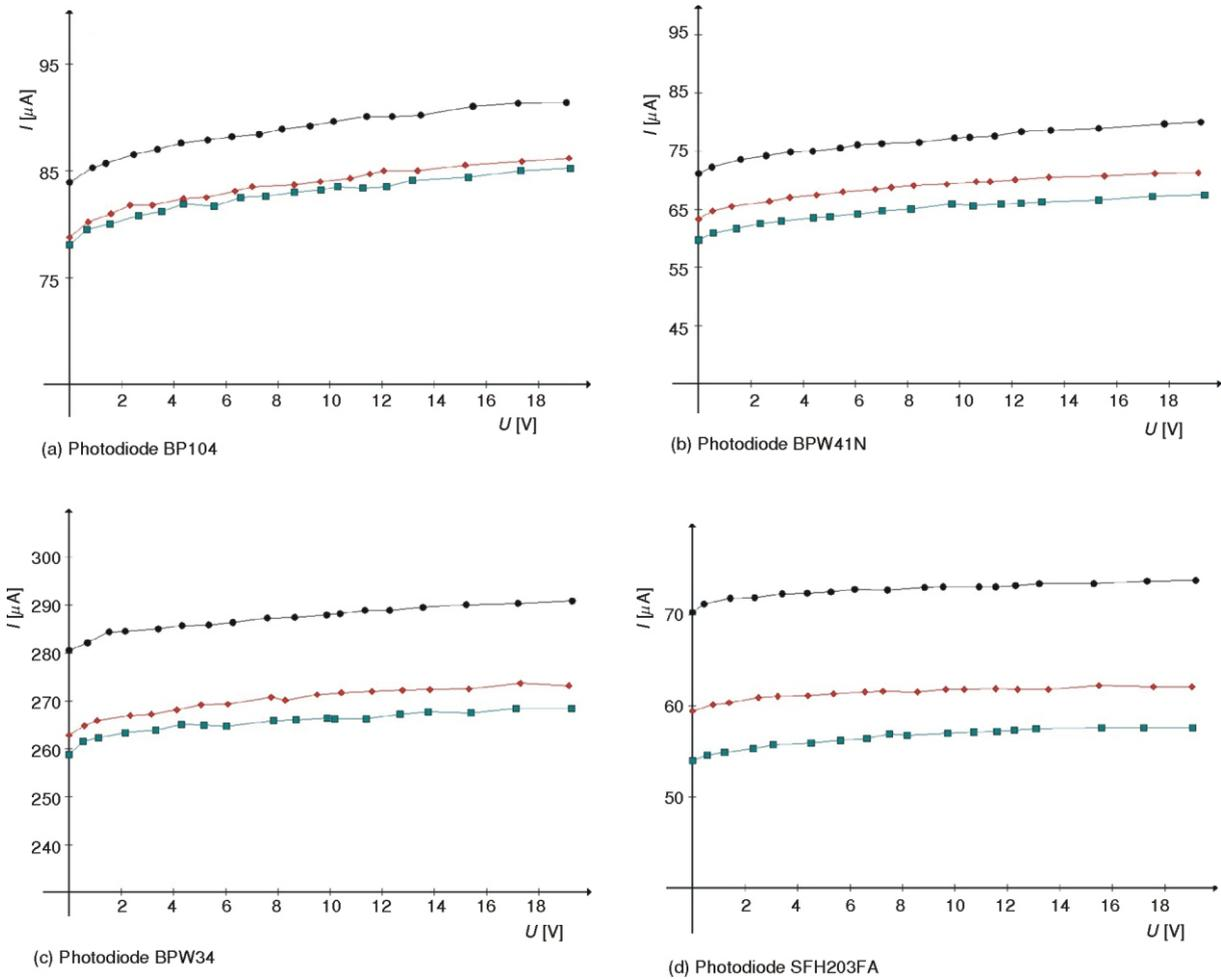
Figure 4. I-V characteristics of the new photodiodes (reverse biased) before and after the neutron irradiation
