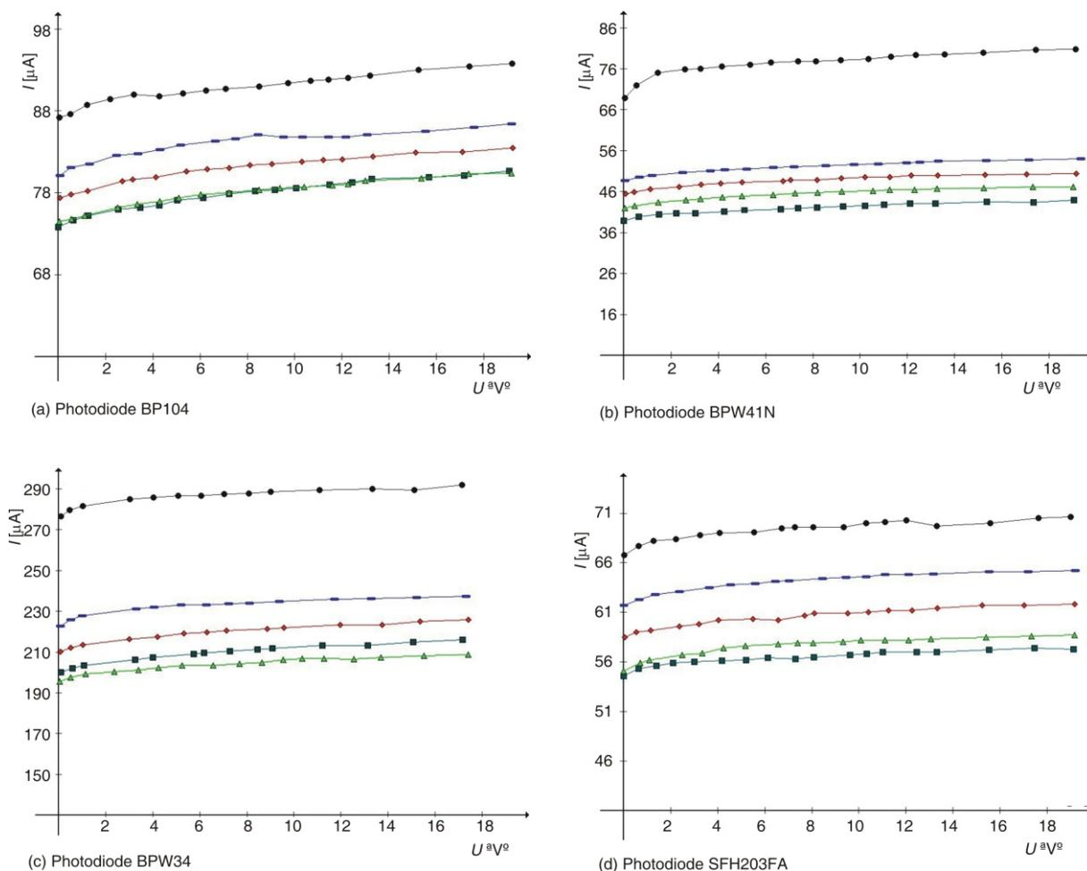
**Figure 2. I-V characteristics of the reverse biased photodiodes before and after every step of the irradiation**
