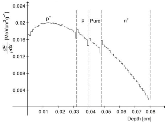
Figure 3. Depth dose distribution in semiconductor (PIN photodiode)
