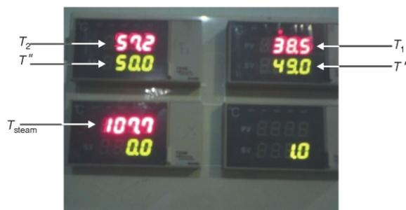
**Figure 3.** A typical temperature over a working session of the TRR, showing real values and set points
