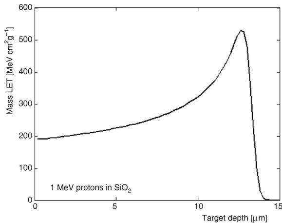
**Figure 5.** Plot of the mass LET for 1 MeV protons along the depth of a 15  $\mu\text{m}$  thick silicon dioxide film. The scale of the energy loss axis is linear, in contrast to figs. 1-4 where it's logarithmic
