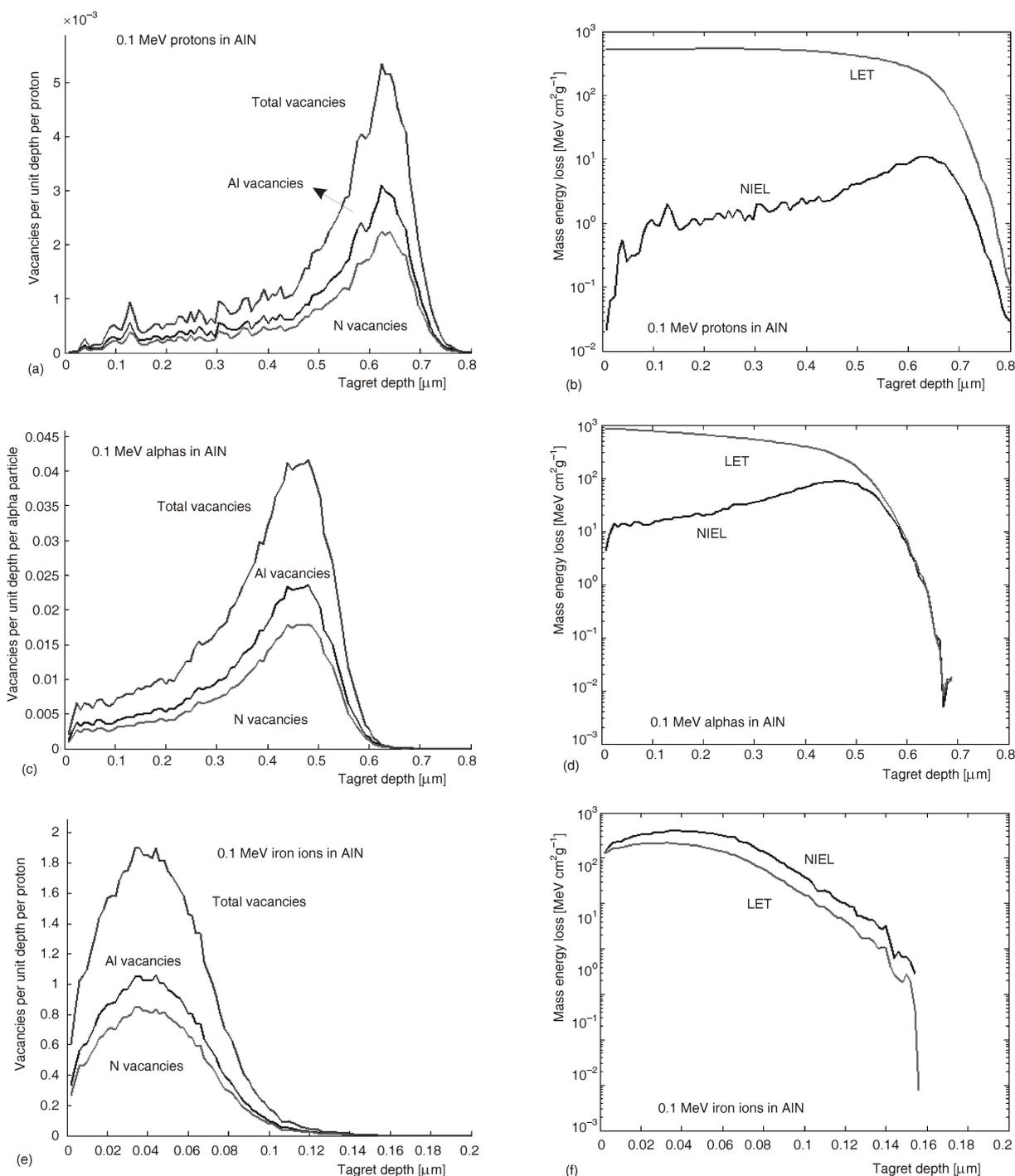
**Figure 2.** Plots of vacancy concentrations and mass energy losses (LET and NIEL divided by material density) along the depth of a aluminum nitride (AlN) insulating film. The results were obtained from simulations of  $10^4$  proton histories (a) and (b),  $10^4$  alpha particle histories (c) and (d), and  $10^3$  iron ion histories (e) and (f), which included subcascades of recoiling silicon and oxygen atoms. The energy of incident heavy charged particles is 0.1 MeV in all cases.
