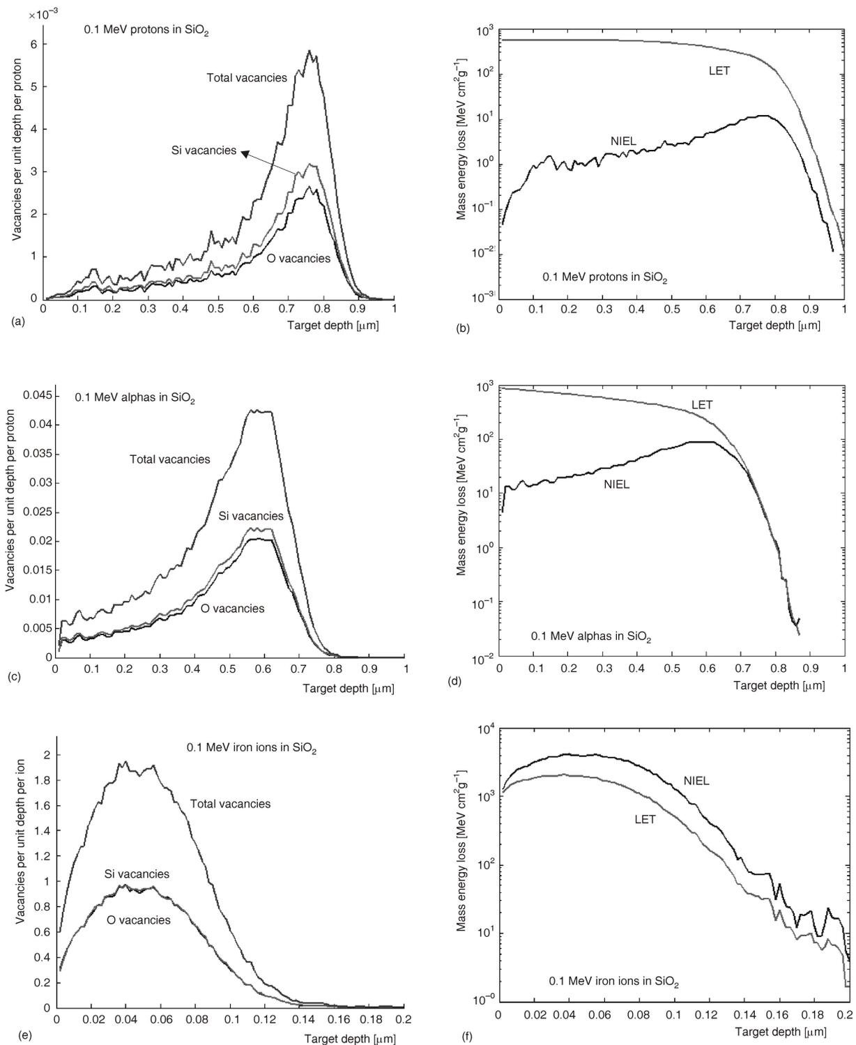
**Figure 1.** Plots of vacancy concentrations and mass energy losses (LET and NIEL divided by material density) along the depth of a silicon dioxide (SiO<sub>2</sub>) insulating film. The results were obtained from simulations of  $10^4$  proton histories (a) and (b),  $10^4$  alpha particle histories (c) and (d), and  $10^3$  iron ion histories (e) and (f), which included subcascades of recoiling silicon and oxygen atoms. The energy of incident heavy charged particles is 0.1 MeV in all cases.
