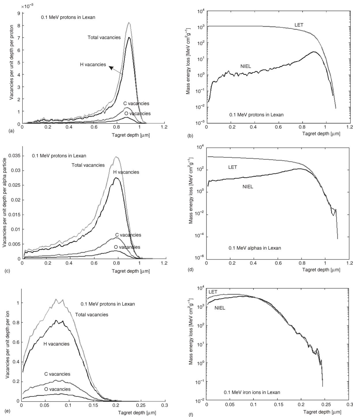
**Figure 4.** Plots of vacancy concentrations and mass energy losses (LET and NIEL divided by material density) along the depth of a lexan (polycarbonate) insulating film. The results were obtained from simulations of  $10^4$  proton histories (a) and (b),  $10^4$  alpha particle histories (c) and (d), and  $10^3$  iron ion histories (e) and (f), which included subcascades of recoiling silicon and oxygen atoms. The energy of incident heavy charged particles is 0.1 MeV in all cases.
