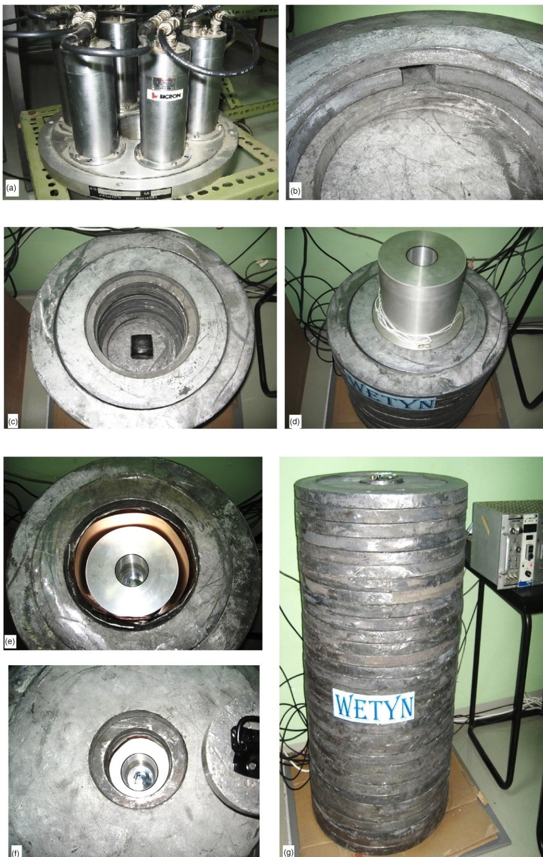
Figure 2. (a) The 9" 9" NaI(Tl) detector with photomultipliers up; (b) the 3 cm wide path for cables; (c) the 2 cm narrower rings around the photomultipliers as a holder for the whole detector; (d) the 9" 9" NaI(Tl) well-type detector outside the shield; (e) the Sn and Cu layers; (f) the opening for samples changing; (g) the assembled shield
