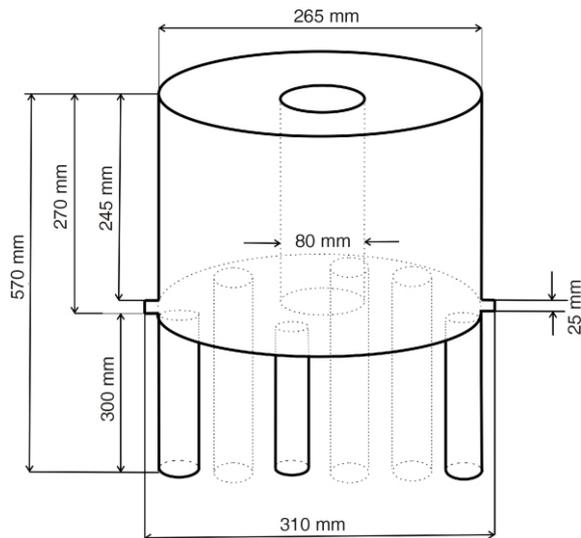
**Figure 1. Schematic diagram of the  $^{99}\text{NaI(Tl)}$  detector with 6 photomultipliers**
