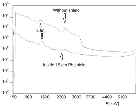
**Figure 3. The  $^{99}\text{Tc}$  NaI(Tl) spectrum without the shield and inside the 15 cm Pb shield (log scale)**
