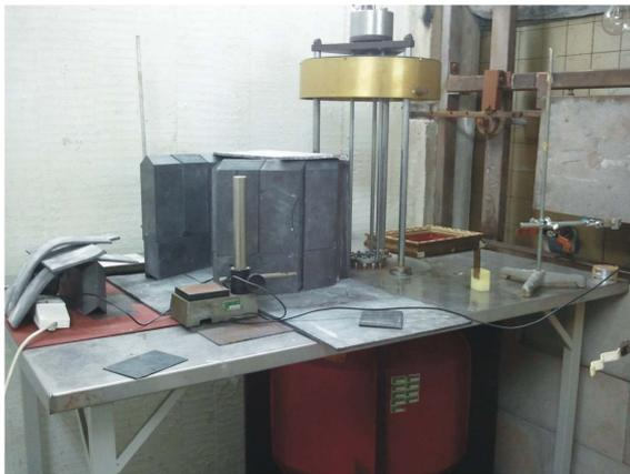
**Figure 3. The lead collimation system**
