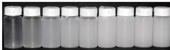
**Figure 13.** Calibrating series made of MAGAT gel imaged after radiation. The opacity change due to growing radiation dose can easily be seen by eyes
