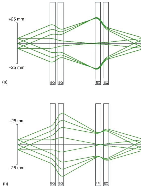
**Figure 2. The beam optics of the first sub-section in the bending plane (a) and the beam optics of the first sub-section in the vertical plane (b)**
