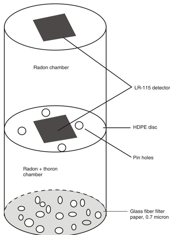
Figure 2. Pinhole based radon-thoron dosimeter used for the study
