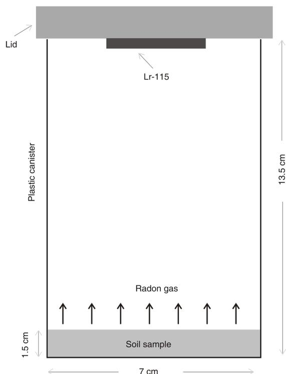
Figure 3. Canister used during the study
