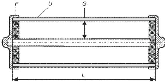
Figure 1. Segment of a GM counter chamber
