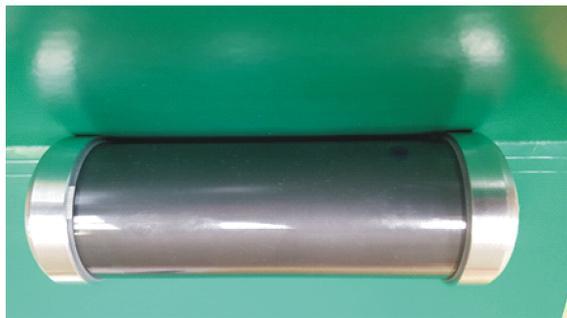
Figure 3. Model of a one segment GM counter
