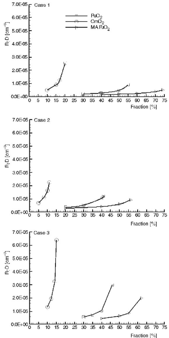
**Figure 5. Variations of  $^{233}\text{U}$  breeding density with the  $\text{TRUO}_2$  fraction in the fuel mixtures (Th,  $\text{TRUO}_2$ )**
