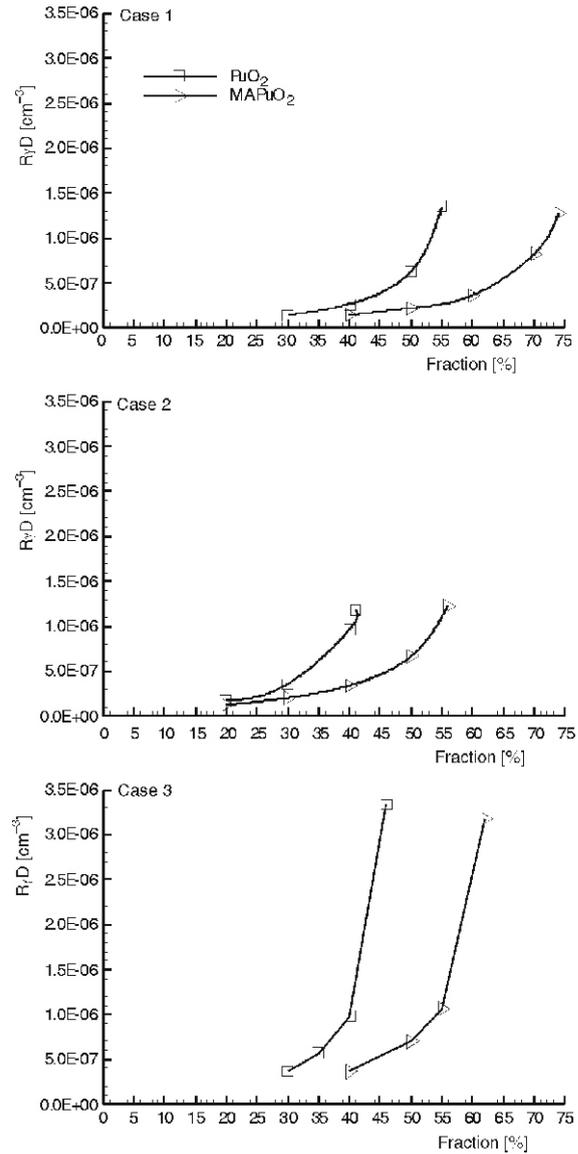
**Figure 6(b).** Variations of <sup>239</sup>Pu breeding density with the TRUO<sub>2</sub> fraction in the fuel mixtures (Th, TRU)O<sub>2</sub> at the transmutation zone
