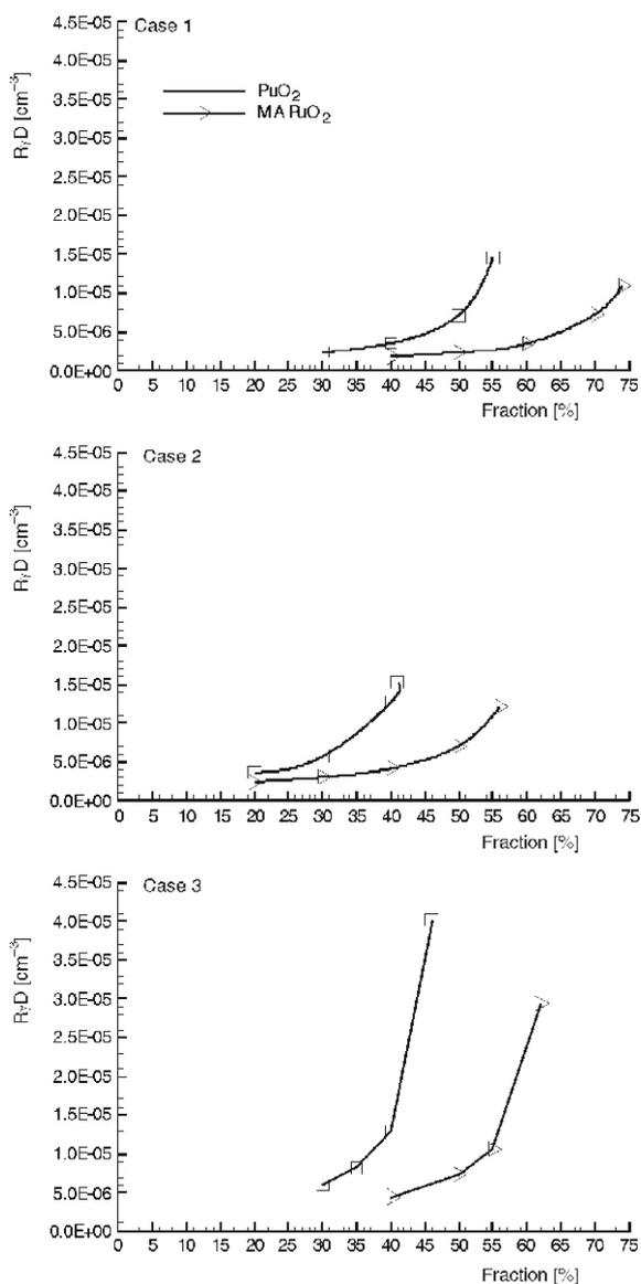
Figure 7. Variations of <sup>241</sup>Pu breeding density with the TRUO<sub>2</sub> fraction in the fuel mixtures (Th, TRU)O<sub>2</sub>
