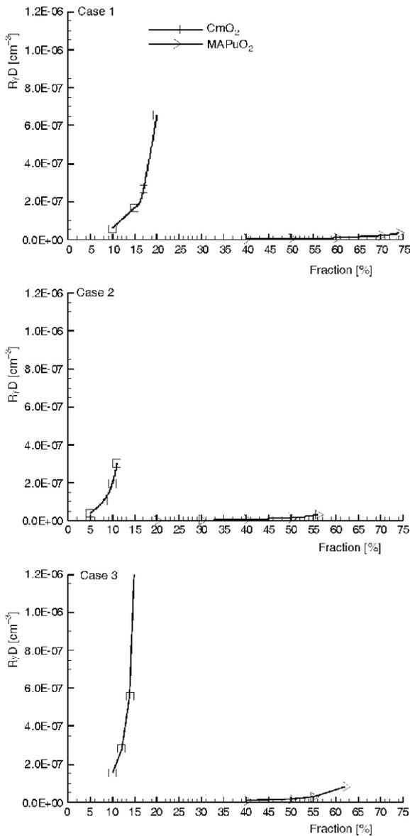
Figure 9. Variations of  $^{243}\text{Cm}$  breeding density with the  $\text{TRUO}_2$  fraction in the fuel mixtures  $(\text{Th}, \text{TRU})\text{O}_2$
