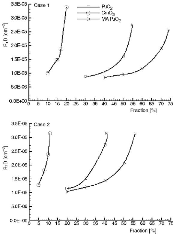
**Figure 6(a).** Variations of <sup>239</sup>Pu breeding density with the TRUO<sub>2</sub> fraction in the fuel mixtures (Th, TRU)O<sub>2</sub> at the inner sub-zone of the target zone
