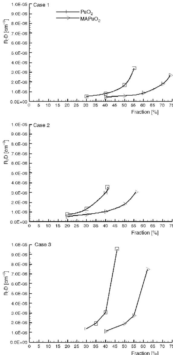
Figure 8. Variatons of <sup>243</sup>Pu breeding density with the TRUO<sub>2</sub> fraction in the fuel mixtures (Th, TRU)O<sub>2</sub>
