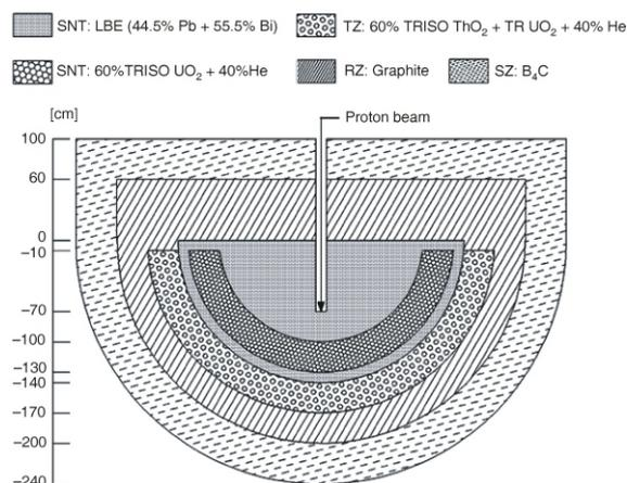
**Figure 1. Cross-section of the investigated ADS (SNT: spallation neutron target, TZ: transmutation zone, RZ: reflector zone, SZ: shield zone)**
