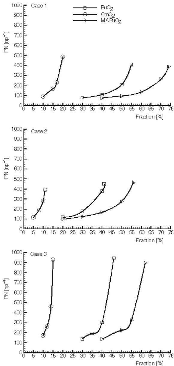
Figure 3. Variations of the neutron production number with the TRUO<sub>2</sub> fraction in the fuel mixtures (Th, TRU)O<sub>2</sub>
