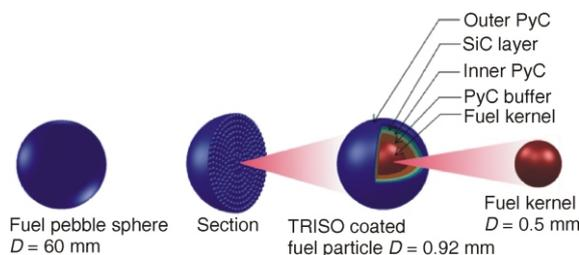
**Figure 2. Fuel pebble sphere and TRISO coated fuel particle, (PyC: pyrocarbon, SiC: silicon carbide)**
