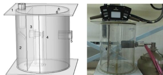
**Figure 2. Set-up employed for the present measurements; 1 – collimator of the X-ray tube, 2 – secondary target, 3 – conical collimator, 4 – sample, 5 – detector collimator, 6 – vacuum pump**
