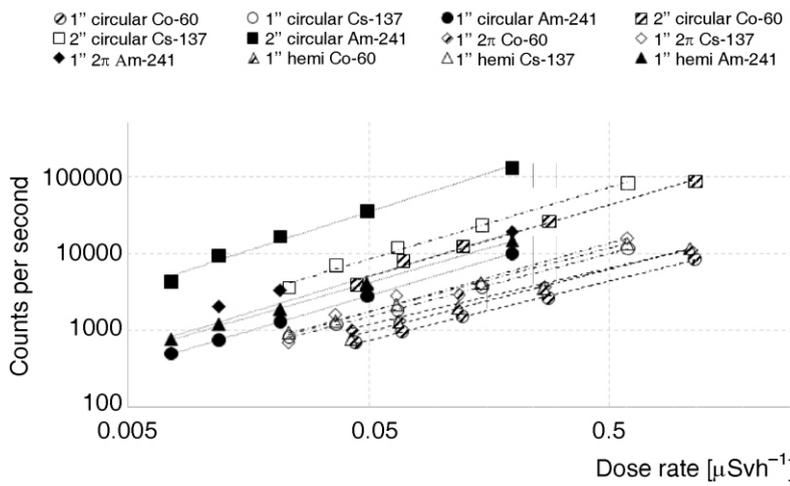
**Figure 5. Detection efficiency of the bar detector (80 cm 10 cm 5 cm) in connection with different types of PMT**
