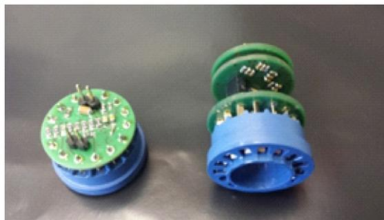
Figure 2. Active divider (left) and active divider in connection with a preamplifier (right)
