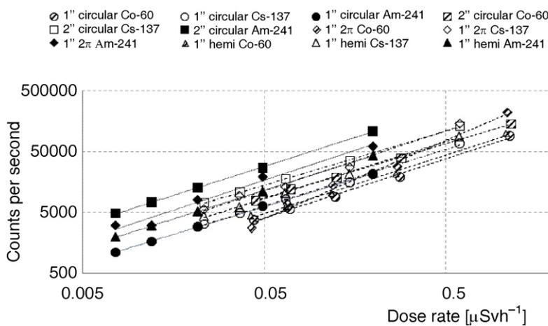
**Figure 6. Detection efficiency of the board detector (100 cm 50 cm 5 cm) in connection with different types of PMT**
