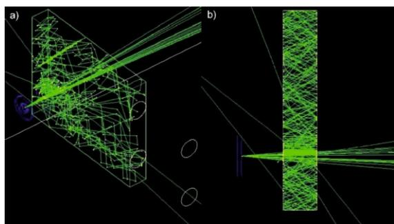
**Figure 7. A visualization showing the tracks of twenty 662 keV photons incident on a polyvinyl toluene detector; (a) oblique view, (b) side view [21]**
