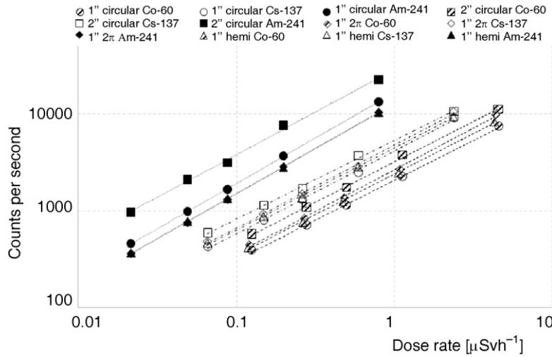
**Figure 4. Detection efficiency of block detector (15 cm 10 cm 5 cm) in connection with different types of PMT**
