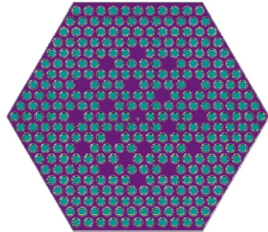
Figure 2. The MCNP plot of VVER fuel assembly
