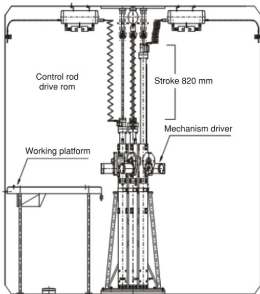
Figure 1. Schematic view of the control rod system
