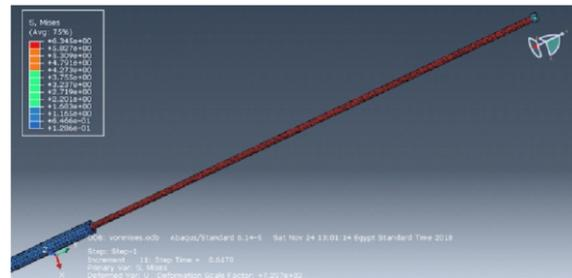
**Figure 6. Von Mises stress at critical impact force  $F = 755.73$  N**
