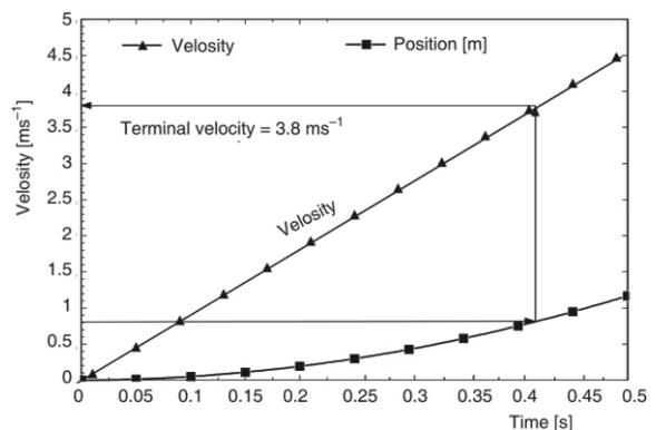
**Figure 8. Control rod drop for 0.5 seconds, solution time**
