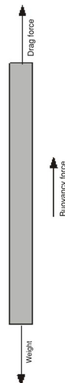
Figure 3. Simple model description of the control rod
