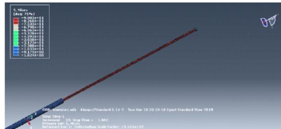
**Figure 7. Von Mises stress at maximum impact force  $F = 6625$  N**
