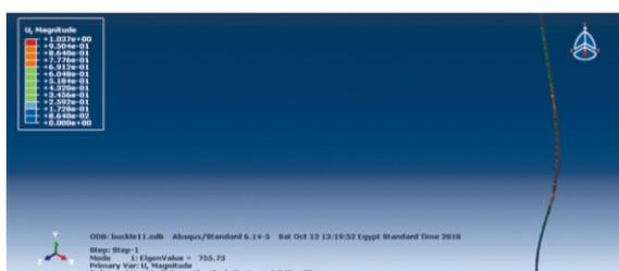
**Figure 5. The ABAQUS buckling deformation at impact force  $F = 755.73$  N**
