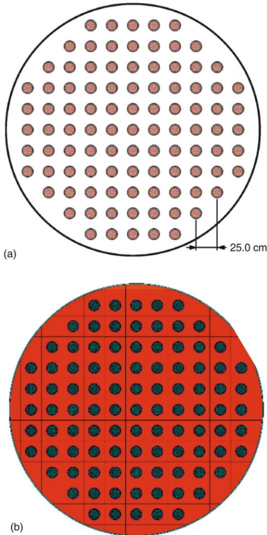
Figure 2. The XY section of the DCA model and comparison with reference models; (a) XY section of the reference model, (b) XY section of DCA models
