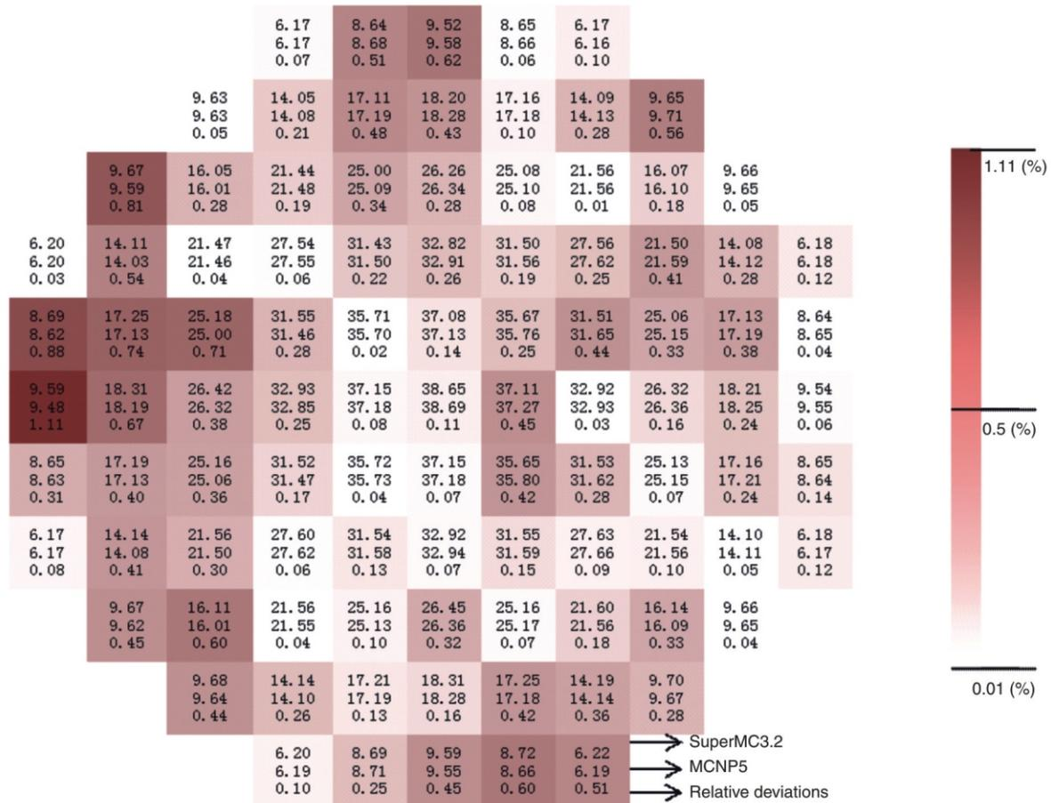
**Figure 4. Results and relative deviations in the radial power distribution between SuperMC3.2 and the reference MCNP results**
