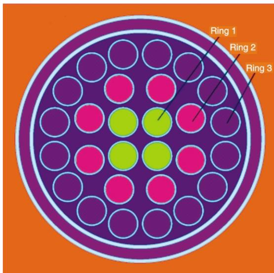
Figure 3. The fuel channel of the DCA reactor
