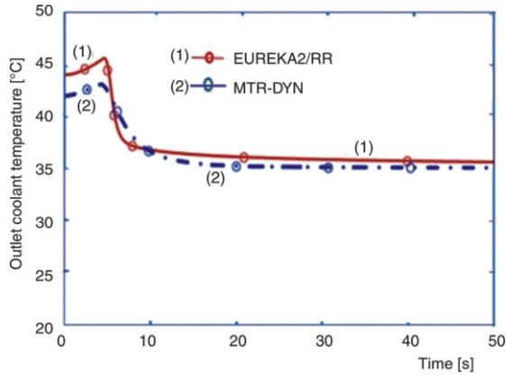
**Figure 10. Outlet coolant flow temperature during the RIA transient**
