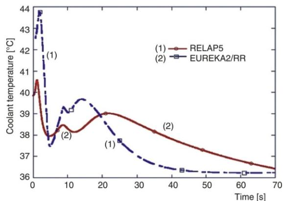
**Figure 14. Outlet coolant flow temperature during the LOFA transient**
