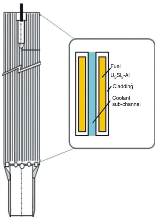
Figure 2. The plate-type fuel element [3]
