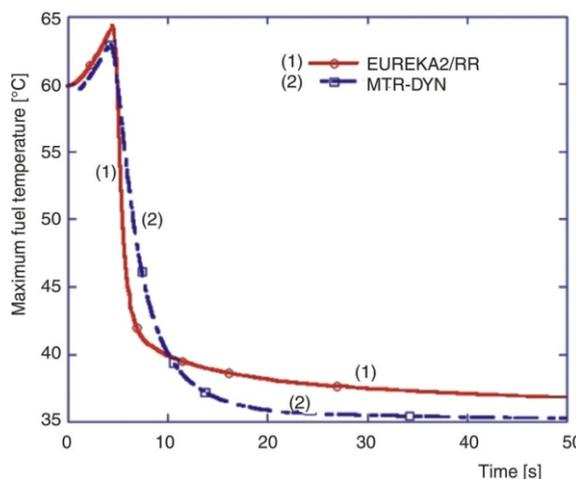
**Figure 8. Maximum fuel temperature profile during RIA transient**
