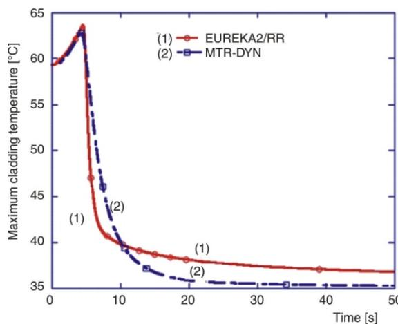
**Figure 9. Maximum cladding temperature profile during RIA transient**
