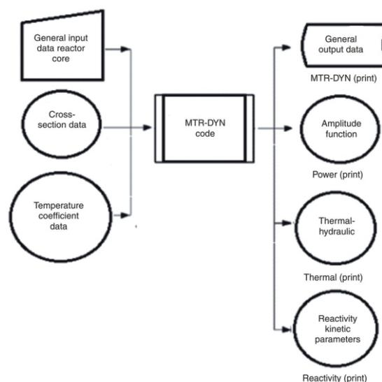
Figure 4. Flow chart diagram for MTR-DYN
