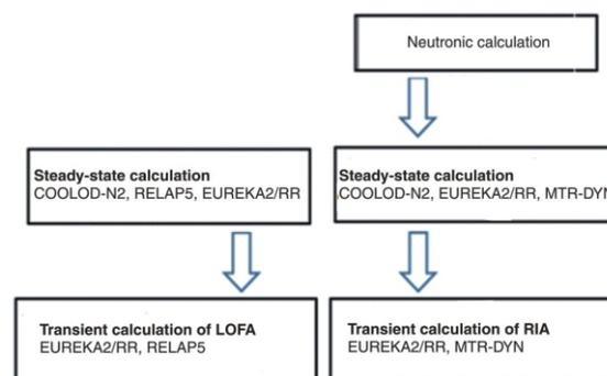
Figure 3. Schematic of steady-state and transient calculation
