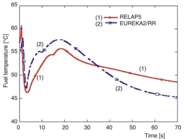
**Figure 12. Maximum fuel temperature profile during LOFA transient**
