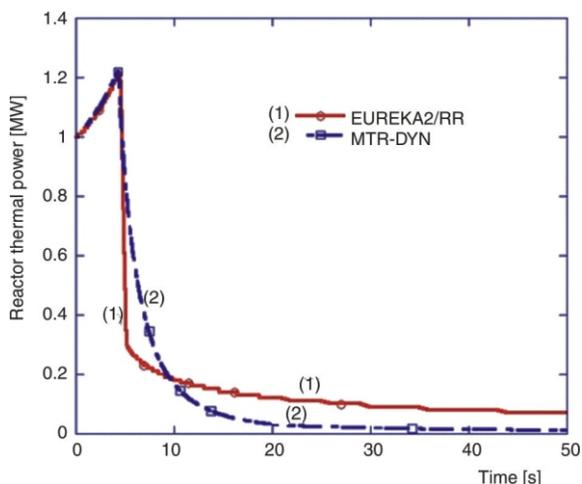
**Figure 7. Reactor power profile during RIA transient**
