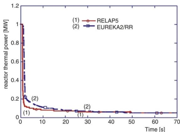
**Figure 11. Power profile during LOFA transient**
