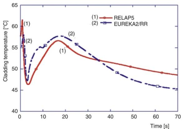
**Figure 13. Maximum cladding temperature profile during LOFA transient**
