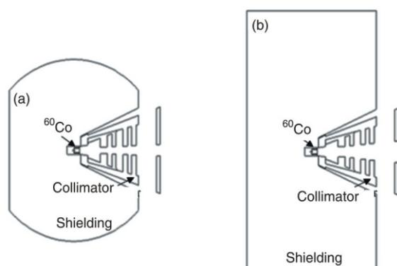
**Figure 2. Geometric structure of  $^{60}\text{Co}$  irradiator for Monte Carlo simulation for (a) vertical axis and (b) lateral axis**
