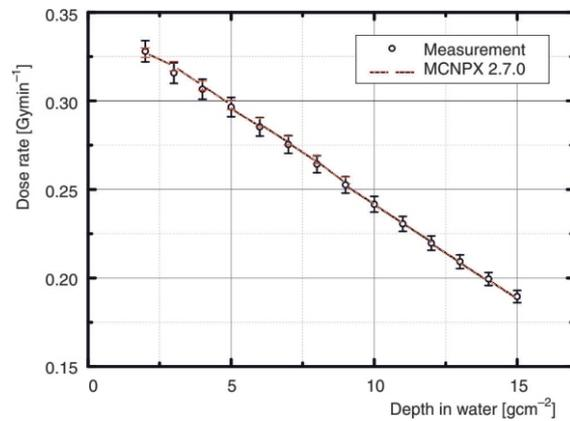
**Figure 5. Comparison of depth profiles for absorbed dose between the measurements and Monte Carlo simulations with gamma field (10 cm × 25 cm field at SCD of 105 cm) in the water phantom**
