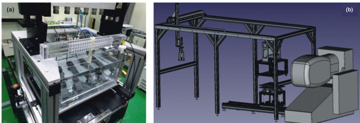
Figure 1. Irradiation system of  $^{60}\text{Co}$  isotope for (a) experimental set-up for absorbed dose in water and (b) geometric structure of water phantom
