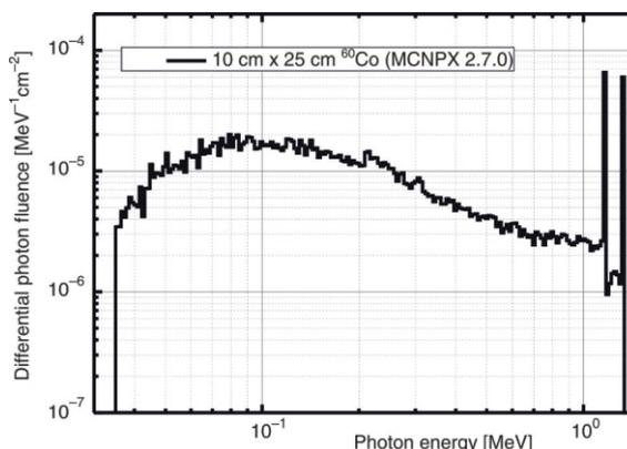
**Figure 3. Differential photon fluence of  $^{60}\text{Co}$  irradiator by Monte Carlo simulation with gamma field ( $10 \text{ cm} \times 25 \text{ cm}$  at SSD of 100 cm) at  $5 \text{ gcm}^{-2}$  depth in the water phantom**
