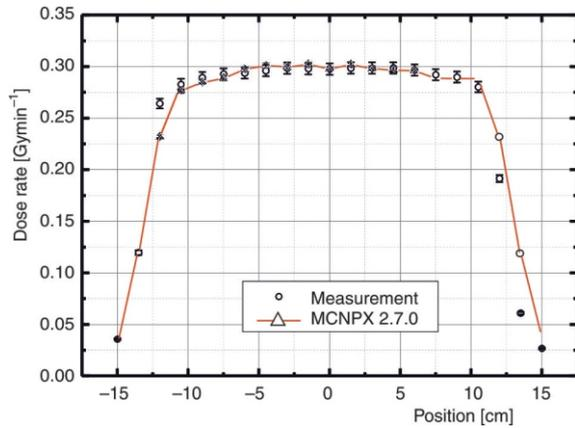
**Figure 4. Comparison of lateral beam profiles for absorbed dose between measurements and Monte Carlo simulations with gamma field (10 cm × 25 cm field at SSD of 100 cm) at 5 gcm<sup>-2</sup> depth in the water phantom**
