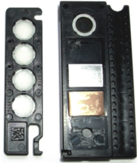
Figure 2. The OSLD components: a slider containing detector elements, and a filtered holder
