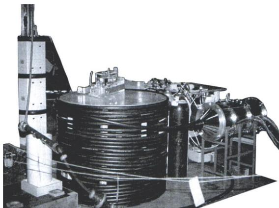
**Figure 3. Cable generator for generating a rise pulse of about 1 ns**
