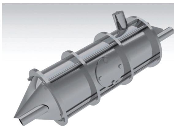
**Figure 4. Model of the horizontal part of the electronic generator with a built-in fast capacitive probe**
