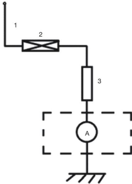
**Figure 6. Experimental scheme: 1 – antenna, 2 – gas-filled surge arrester, 3 – grounding resistance, and 4 – cabin for protection against electromagnetic waves greater than 100 dB**
