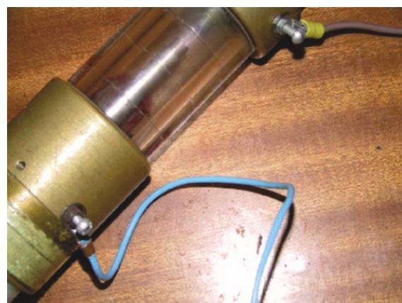
**Figure 7. Flexible model of the gas-filled surge arrester**
