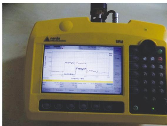
**Figure 5. Non-ionizing electromagnetic radiation field generated by triggering a fusion generator model at a distance of 1 km from the experimental plant**
