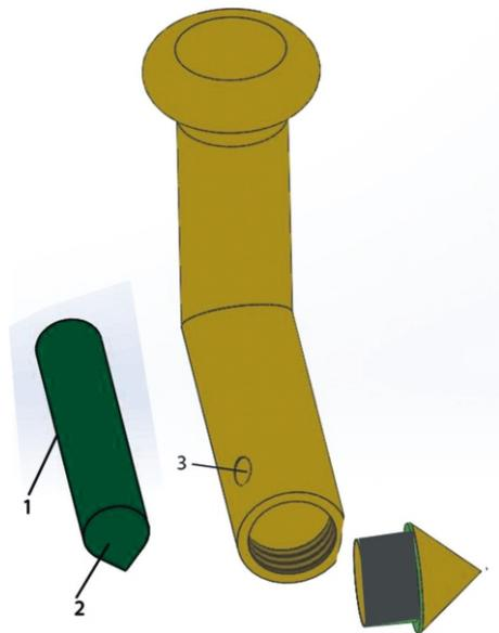
**Figure 1. Electronic generator: 1 – pulse shaping circuit, 2 – 50 Ω waveguide adapter resistance, and 3 – position for setting the measuring and control probe**
