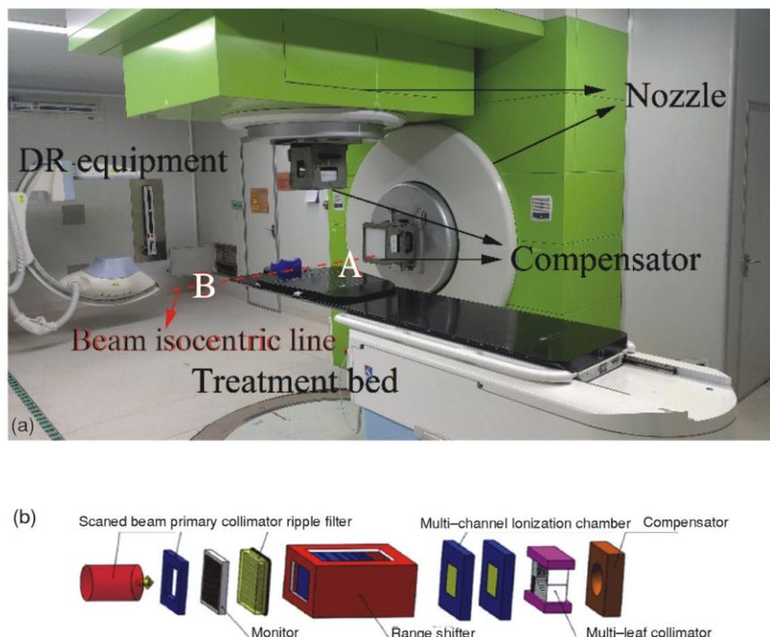
Figure 2. The layout of treatment Room 2; (a) the composition of the treatment room and (b) the composition of the nozzle
