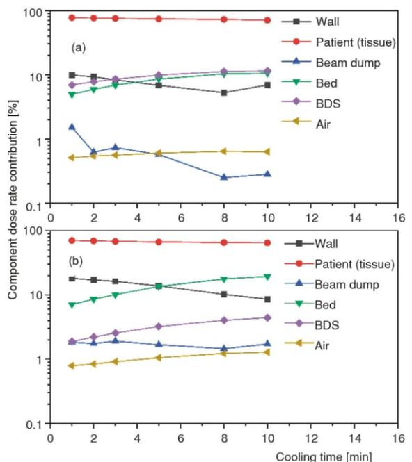
**Figure 5. The dose rate contribution of components with time at Positions A and B for single irradiation; (a) Position A for staff and (b) Position B for staff**
