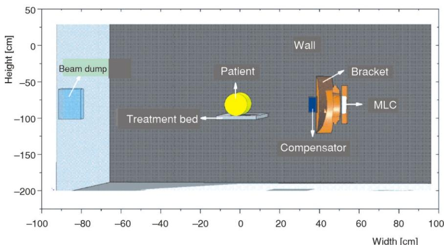
gular (15 cm × 15 cm) on the *X*- and *Y*-axes. An 8 cm × 8 cm × 6 cm rectangle filled with air acted as a grid in the middle of the MLC, and a 8 cm × 7.5 cm cylinder was filled with air to represent the shape of the patient's tumor in the middle of the compensator. The size of the treatment room was 16.98 m × 10.90 m × 4 m and was filled with air. The centers of the MLC, compensator, patient, and beam dump were on the isocentric beam line.
