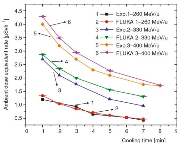
**Figure 4. The dose rates of FLUKA simulation and experimental measurement**
