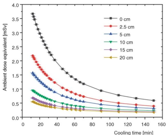
Figure 6. The residual dose at different distances from the compensator with time (400 MeV/u,  $2.4 \cdot 10^7$  pps, irradiation time of 18 minutes)
