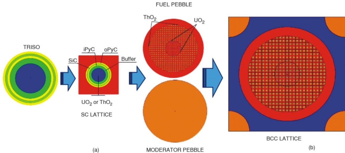
Figure 2. The MCNP6 model for (a) TRISO duplex particle and (b) fuel pebble
