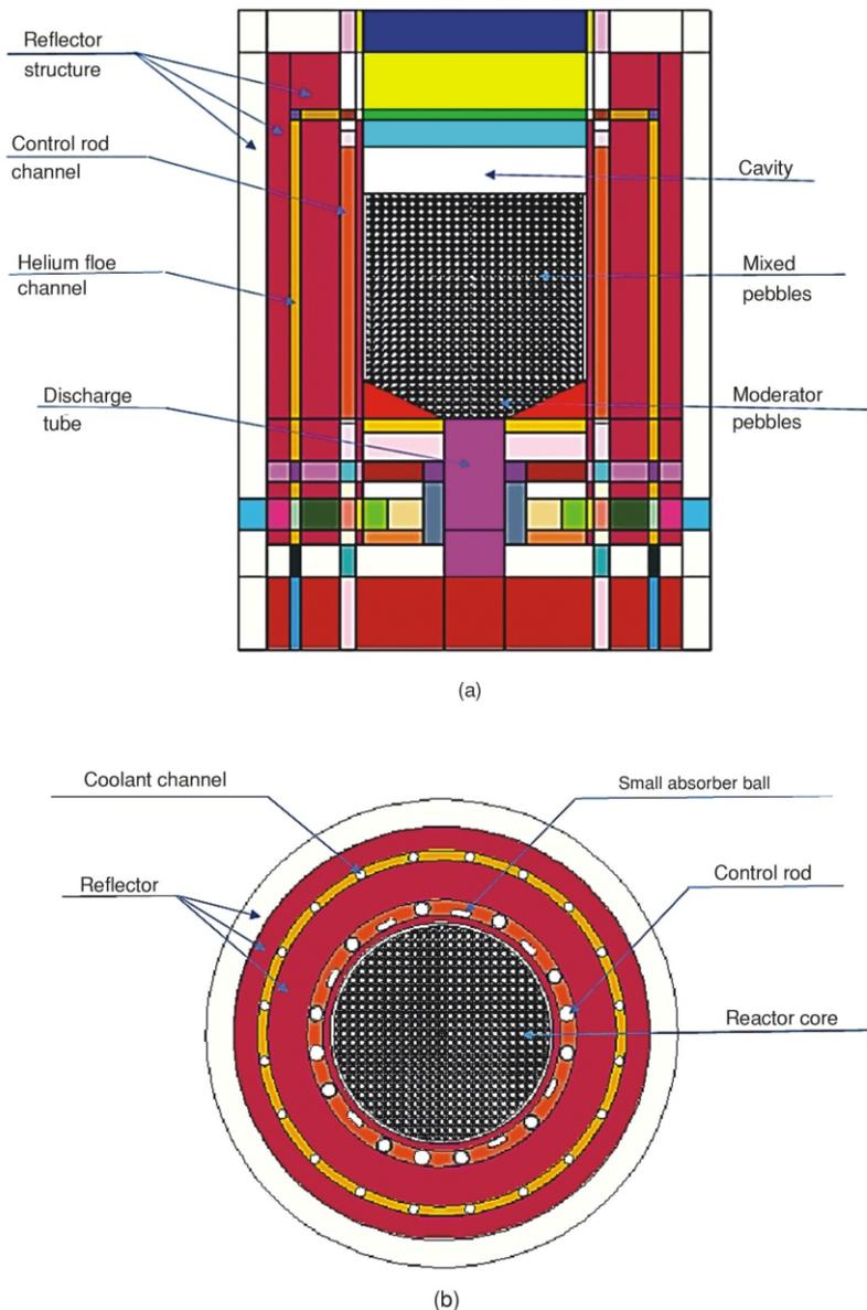
Figure 3. The MCNP6 model for (a) the axial and (b) radial views of the reactor core
