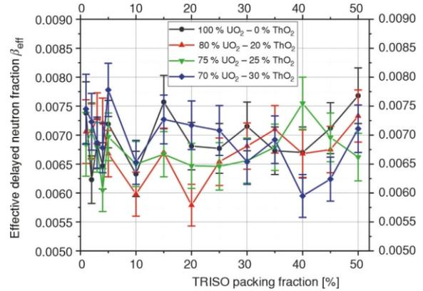
Figure 7. Effective delayed neutron fraction  $\beta_{\text{eff}}$
