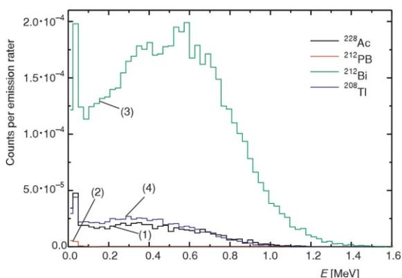
**Figure 1.** The BC404 Response vs. electron energy in counts per emission rate for beta emitters in the thorium chain; (1)  $^{228}\text{Ac}$ , (2)  $^{212}\text{Pb}$ , (3)  $^{212}\text{Bi}$ , and (4)  $^{208}\text{Tl}$
