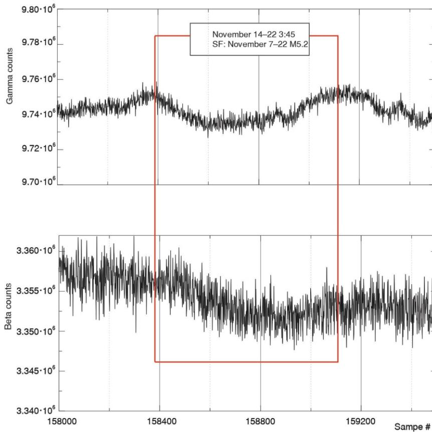
Figure 2. Thorium count-rate dip measured by the gamma detector (up), and the beta detector (down). Information about the relevant SF is provided with the time (UT + 2)
