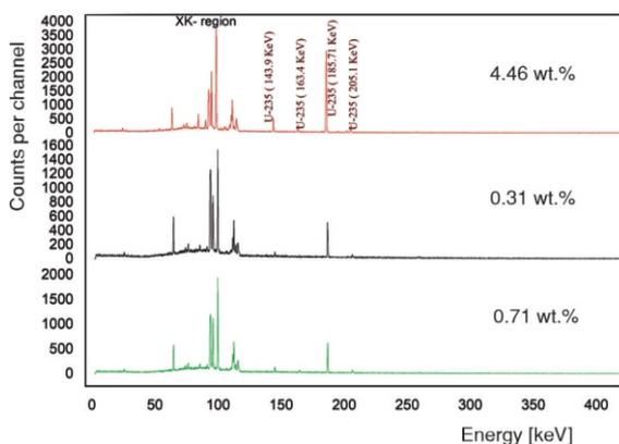
**Figure 2. Gamma spectra of U<sub>3</sub>O<sub>8</sub> oxide samples with various enrichment 0.31 wt.%, 0.71 wt.%, and 4.46 wt.% in the energy region of 0-400 keV**
