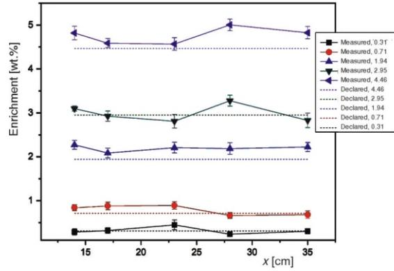
Figure 6. Relation of the enrichment at a different S-D position for different samples
