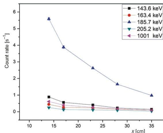
**Figure 8.** Relation of the count rate of the measured CRM2 of 0.71 % at a different S-D distance and different energy lines
