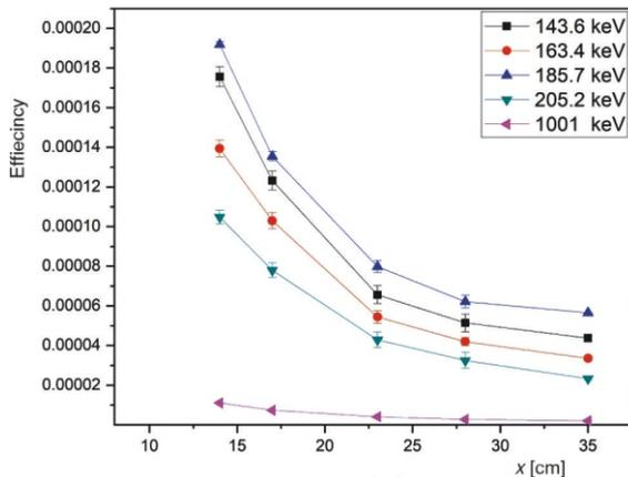
Figure 5. Full energy peak efficiency of the measured CRMs of 4.46% at a different S-D position
