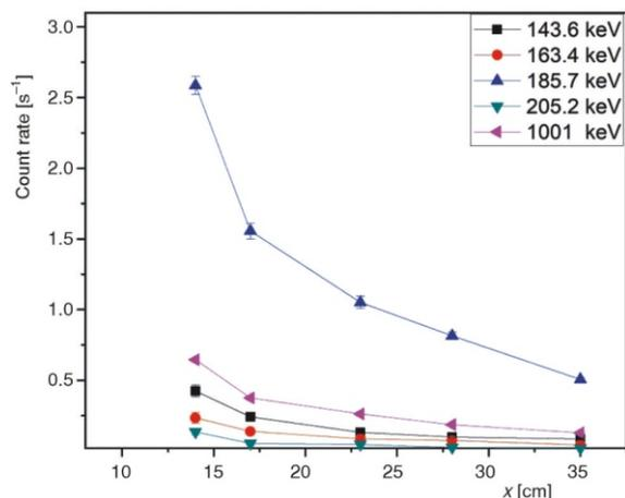
**Figure 7.** Relation of the count rate of the measured CRM1 of 0.31 % at a different S-D distance and different energy lines
