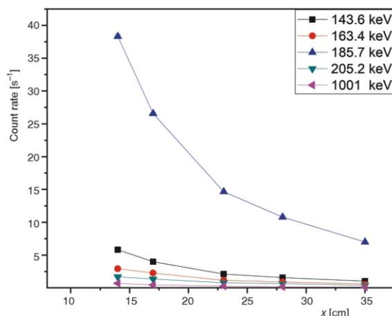
**Figure 9.** Relation of the count rate of the measured CRM5 of 4.46 % at a different S-D distance and different energy lines
