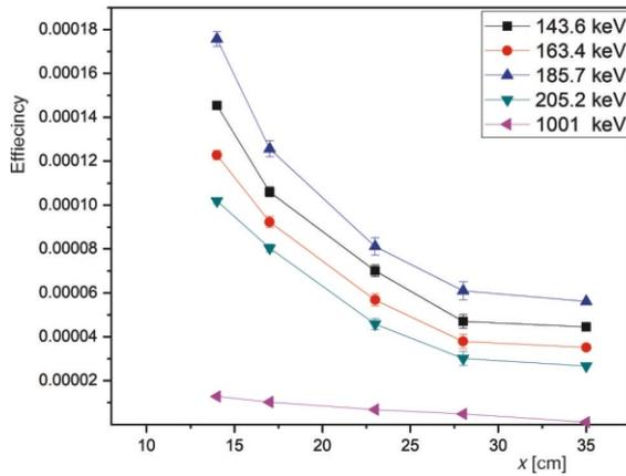
Figure 4. Full energy peak efficiency of the measured CRM2 of 0.71% at a different S-D position
