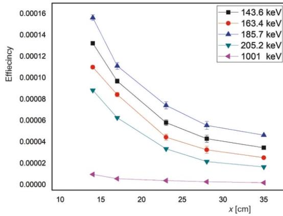
Figure 3. Full energy peak efficiency of the measured CRM1 of 0.31% at a different S-D position and different energy lines
