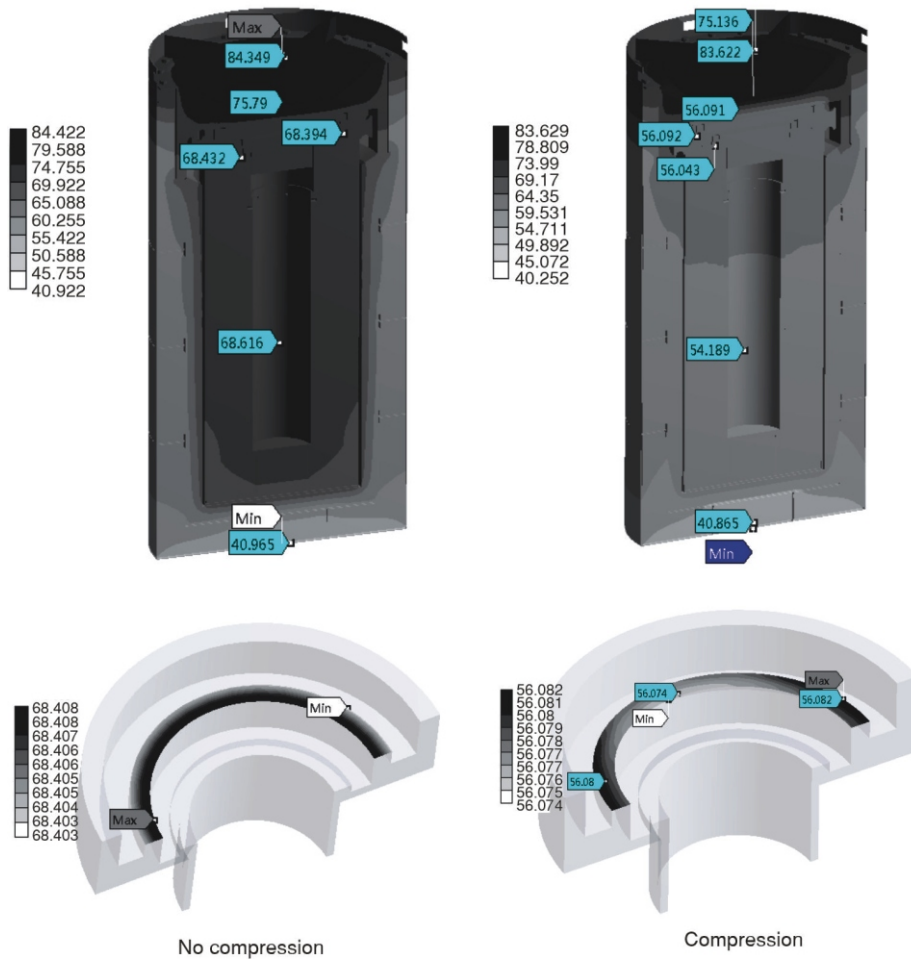
Figure 5. Temperature results of the insulation condition
