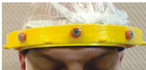
Figure 1. Three TLD secured on a headband in left, middle, and right position, worn on a forehead, approximately 1 cm above the eyebrows
