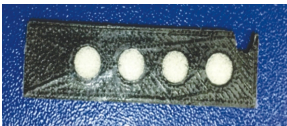
Figure 5. Four-element salt dosimeter
