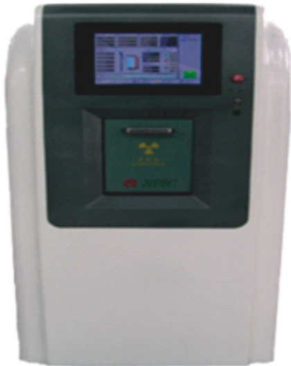
Figure 3. HXFS-IA biological irradiation instrument
