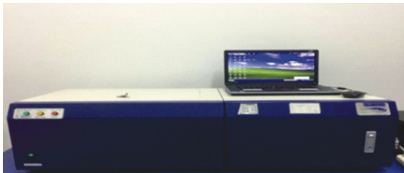
Figure 4. InLight200A photoluminescence personal dose monitoring system
