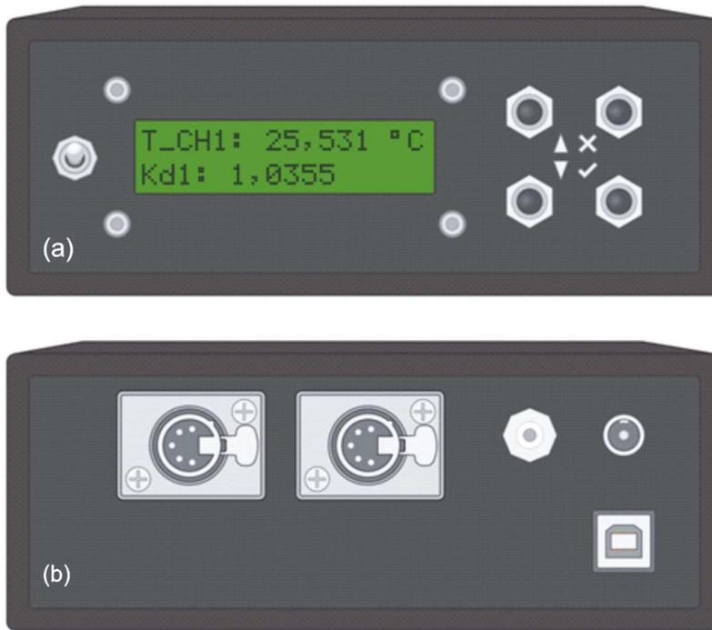
**Figure 2.** Central unit front side with user interface (a) and backside with temperature probe connectors, air inlet, DC power connector, and USB connector (b)
