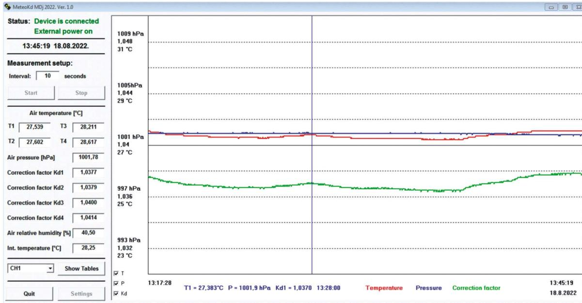
Figure 5. MeteoKd PC software – view of the graph with measured data from a selected probe
