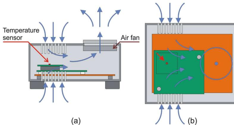
**Figure 3.** Temperature probe enclosure cross-section; air path diagram with position of temperature sensor and air fan side view (a) and top view (b)
