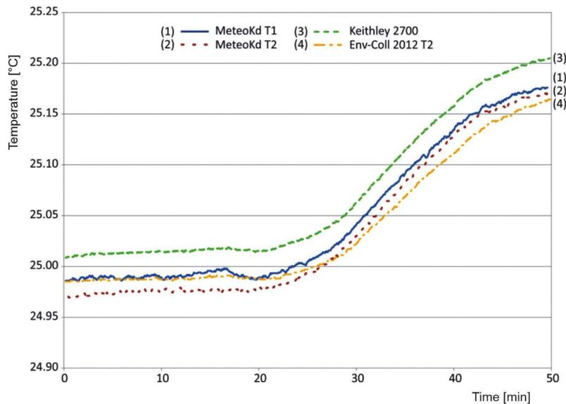
**Figure 10. Comparison of ambient air temperature measurement using three tested instruments**
