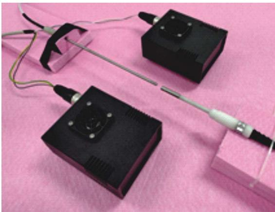
Figure 7. Measurement set-up for ambient temperature measurement
