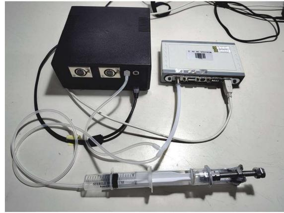
Figure 8. Measurement set-up for air pressure measurement
