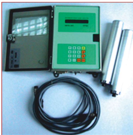
Figure 2. Multifunctional gamma dose rate monitor MFM203 with probes
