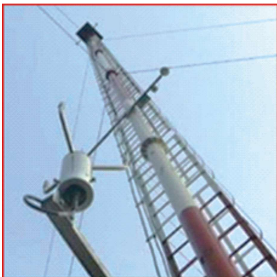
Figure 3. Automated meteorological weather station
